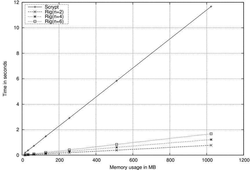
Figure 6: Performance of Rig (at different value of  $n$ ) and Script.
